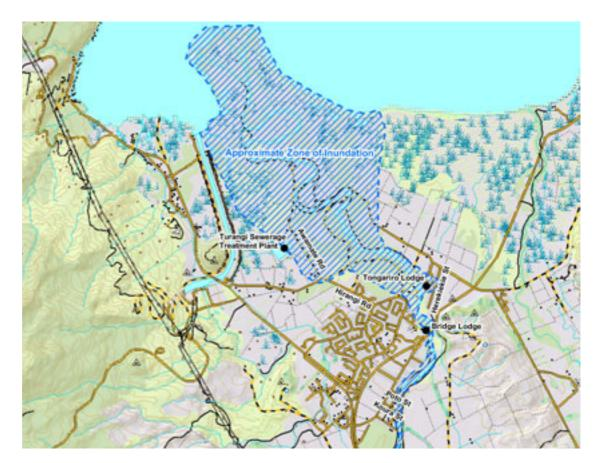
Figure 9: Approximate zone of inundation from Feb. 2004 flood (Bowler, 2004)
