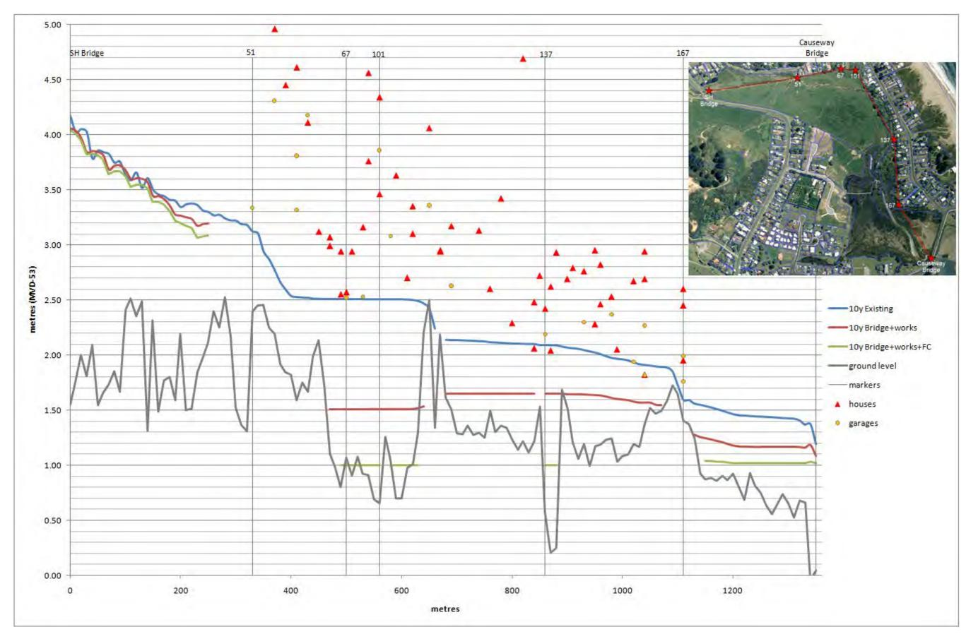
Figure A 27: Ocean Beach Road maximum flood level profiles for existing, current scheme works (partial stopbank), and proposed future works (full stopbank -FC) – 10% AEP (10y ARI).
