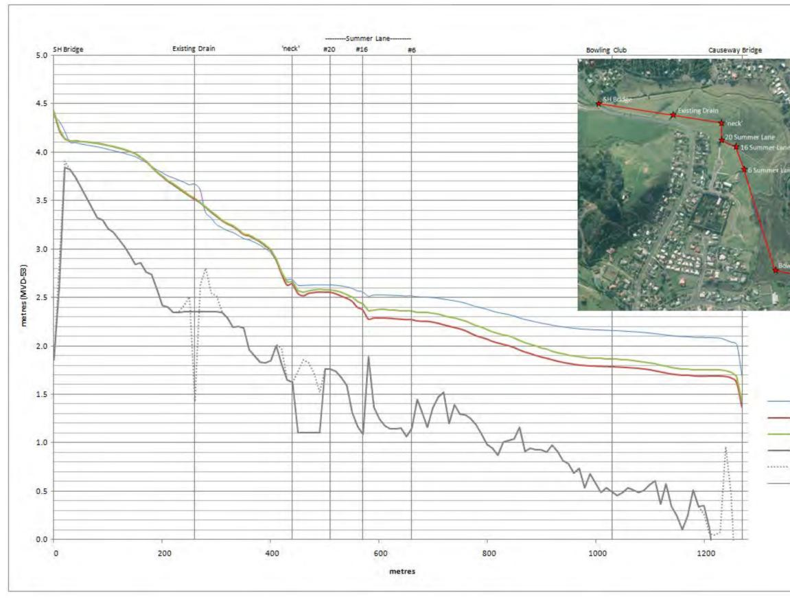
Figure A 39: Right bank floodplain maximum flood level profiles for existing, current scheme works (partial stopbank), and proposed future works (full stopbank -FC) – CC1%AEP (CC100y ARI).
