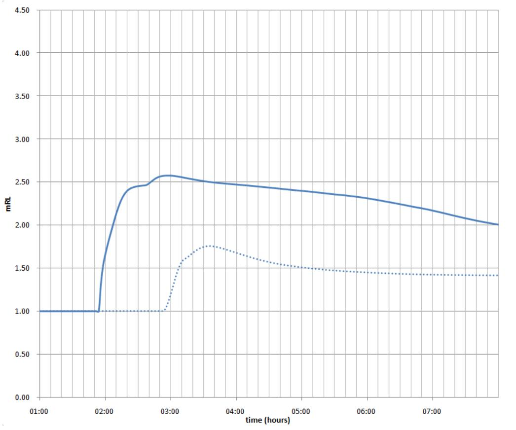
Figure A 50: Right Reduction in flood inundation times during 2% AEP (50y ARI) event for existing and proposed works at #101 Ocean Beach Road.
