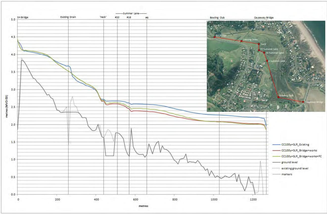
Figure A 40: Right bank floodplain maximum flood level profiles for existing, current scheme works (partial stopbank), and proposed future works (full stopbank -FC) – CC1%AEP+SLR (CC100y ARI+SLR).
