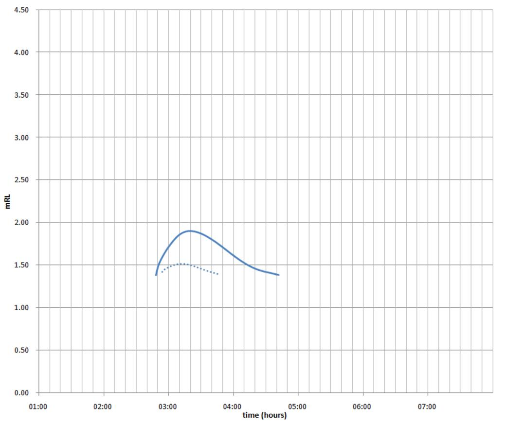
Figure A 52: Right Reduction in flood inundation times during 2% AEP (50y ARI) event for existing and proposed works at #167 Ocean Beach Road.
