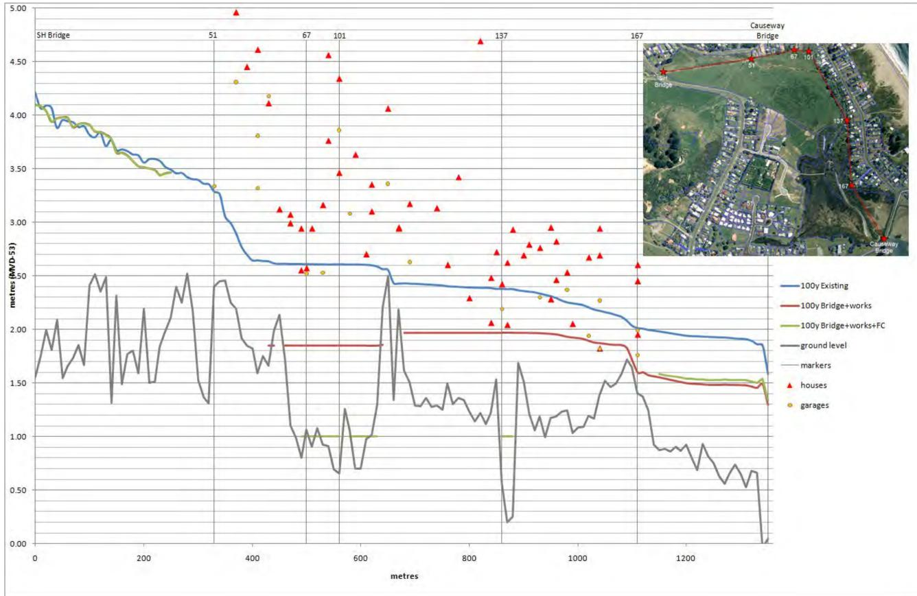
Figure A 30: Ocean Beach Road maximum flood level profiles for existing, current scheme works (partial stopbank), and proposed future works (full stopbank -FC) – 1%AEP (100y ARI).
