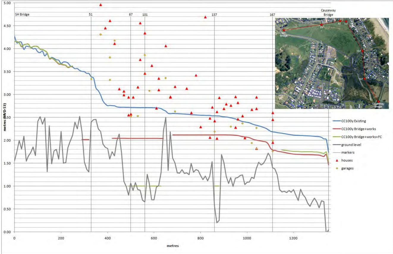
Figure A 31: Ocean Beach Road maximum flood level profiles for existing, current scheme works (partial stopbank), and proposed future works (full stopbank) – CC1%AEP (CC100y ARI).
