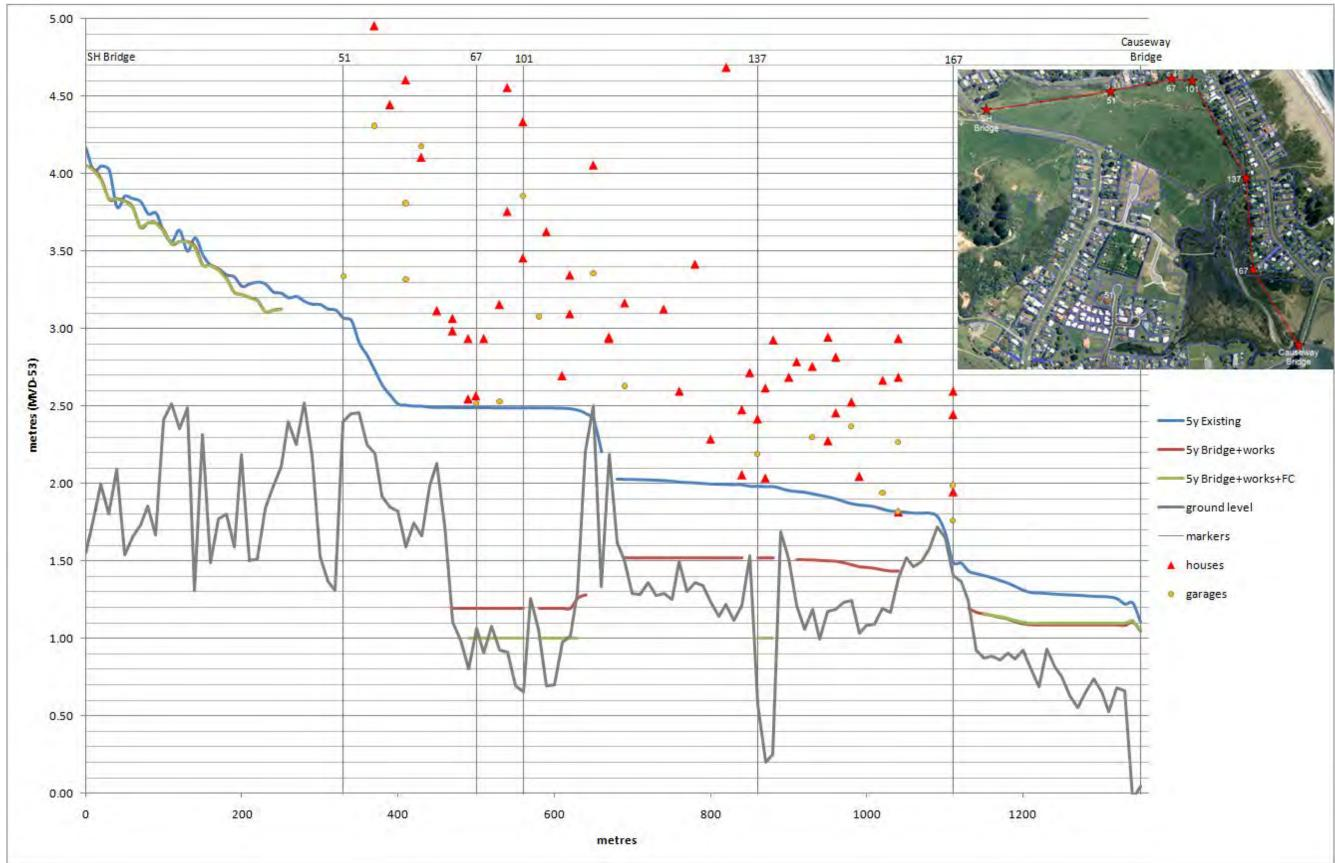
Figure A 26: Ocean Beach Road maximum flood level profiles for existing, current scheme works (partial stopbank), and proposed future works (full stopbank -FC) – 20% AEP (5y ARI).
