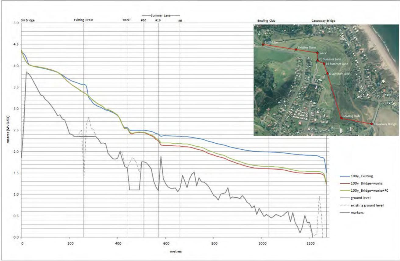
Figure A 38: Right bank floodplain maximum flood level profiles for existing, current scheme works (partial stopbank), and proposed future works (full stopbank -FC) – 1%AEP (100y ARI).
