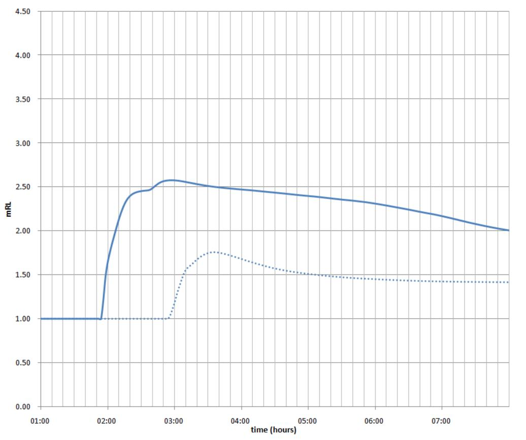
Figure A 49: Reduction in flood inundation times during 2% AEP (50y ARI) event for existing and proposed works at #67 Ocean Beach Road.
