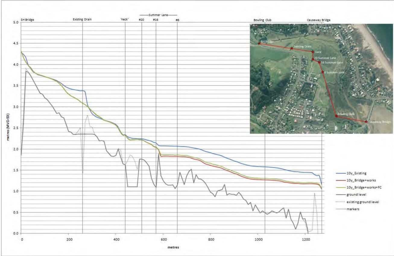
Figure A 35: Right bank floodplain maximum flood level profiles for existing, current scheme works (partial stopbank), and proposed future works (full stopbank -FC) – 10% AEP (10y ARI).
