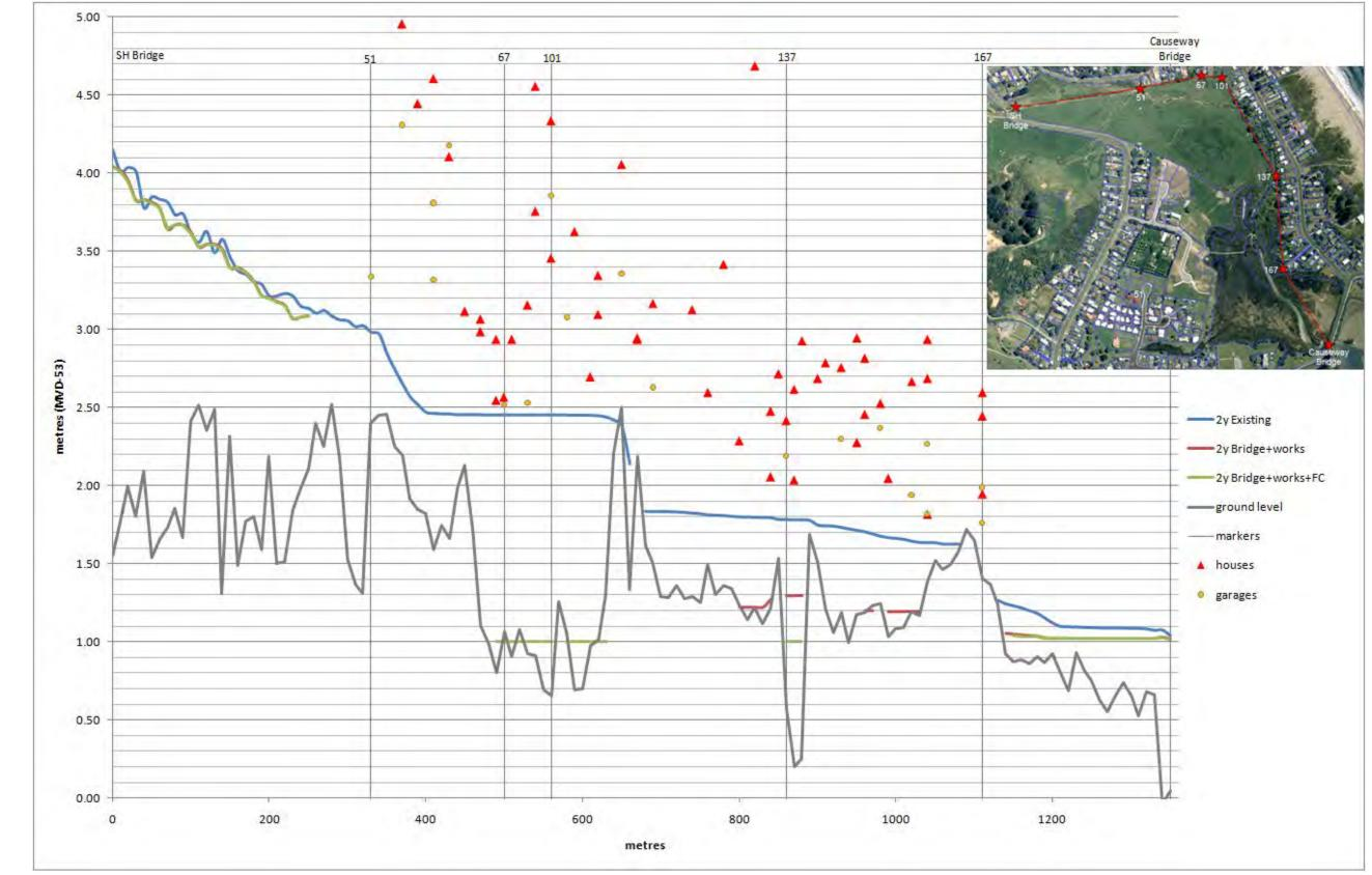
Figure A25 to A32 - Flood level profiles versus floor levels for left bank floodplain on Ocean Beach Road.
