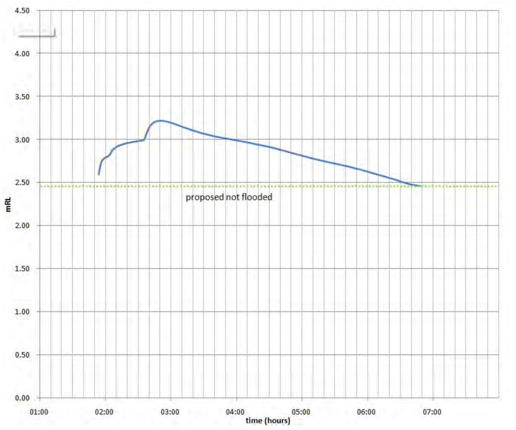
Figure A 48: Reduction in flood inundation times during 2% AEP (50y ARI) event for existing and proposed works at #51 Ocean Beach Road.
