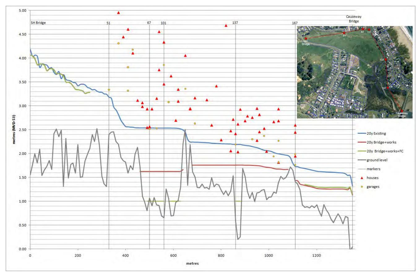
Figure A 28: Ocean Beach Road maximum flood level profiles for existing, current scheme works (partial stopbank), and proposed future works (full stopbank -FC) – 5% AEP (20y ARI).
