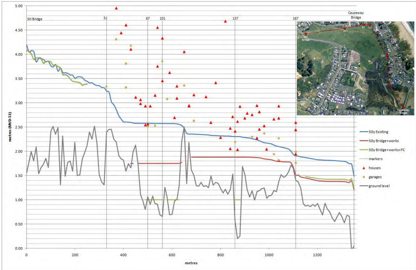
Figure A 29: Ocean Beach Road maximum flood level profiles for existing, current scheme works (partial stopbank), and proposed future works (full stopbank -FC) – 2% AEP (50y ARI).
