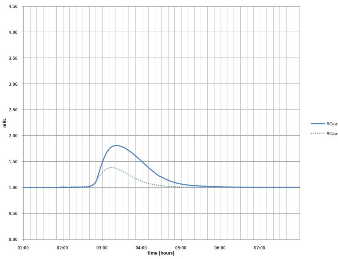
Figure A 53: Reduction in flood inundation times during 2%AEP (50y ARI) event for existing and proposed works at causeway.
