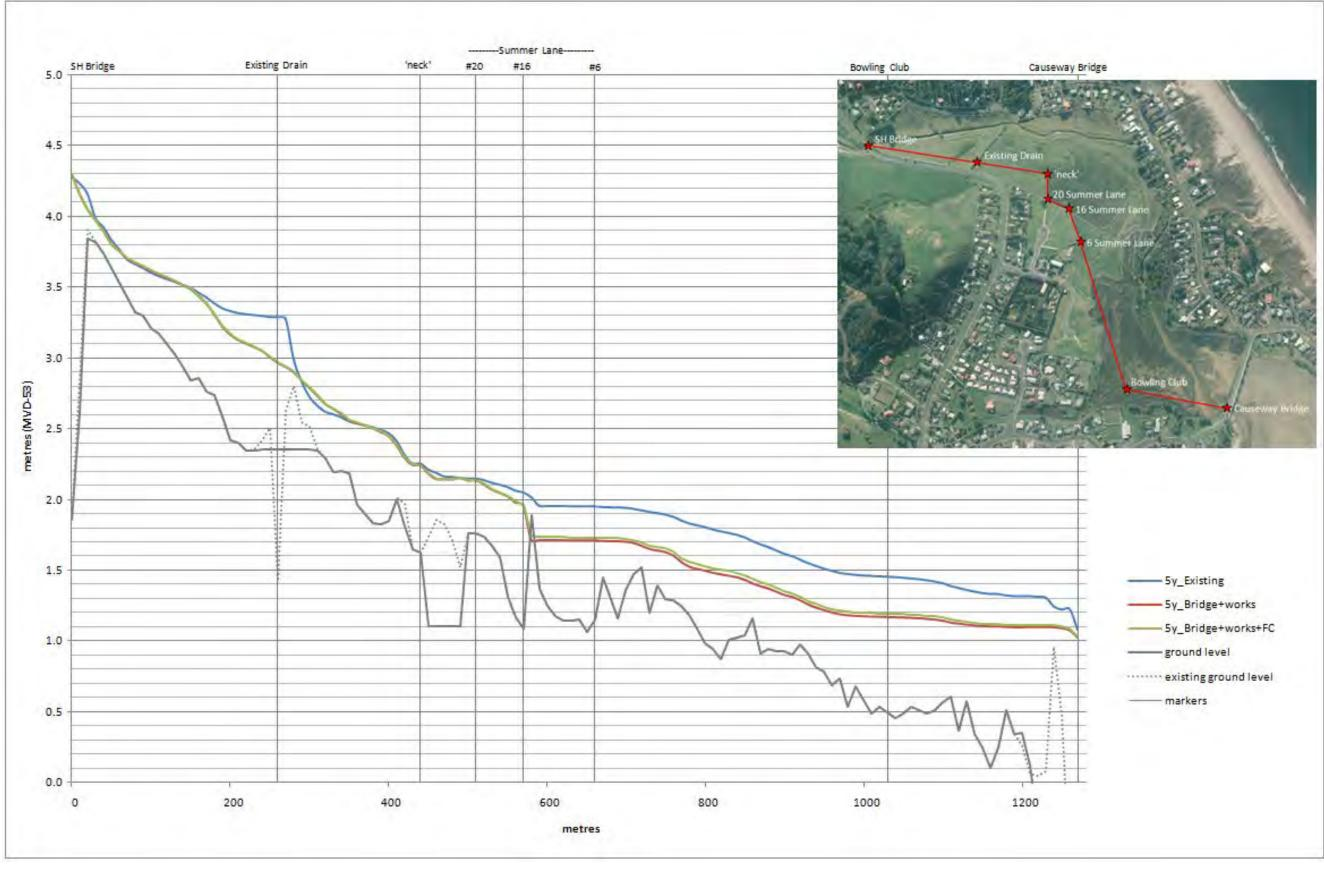
Figure A 34: Right bank floodplain maximum flood level profiles for existing, current scheme works (partial stopbank), and proposed future works (full stopbank -FC) – 20% AEP (5y ARI).
