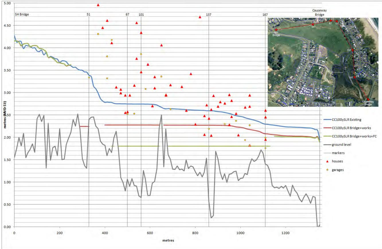
Figure A 32: Ocean Beach Road maximum flood level profiles for existing, current scheme works (partial stopbank), and proposed future works (full stopbank -FC) – CC1%AEP+SLR (CC100y ARI+SLR).
