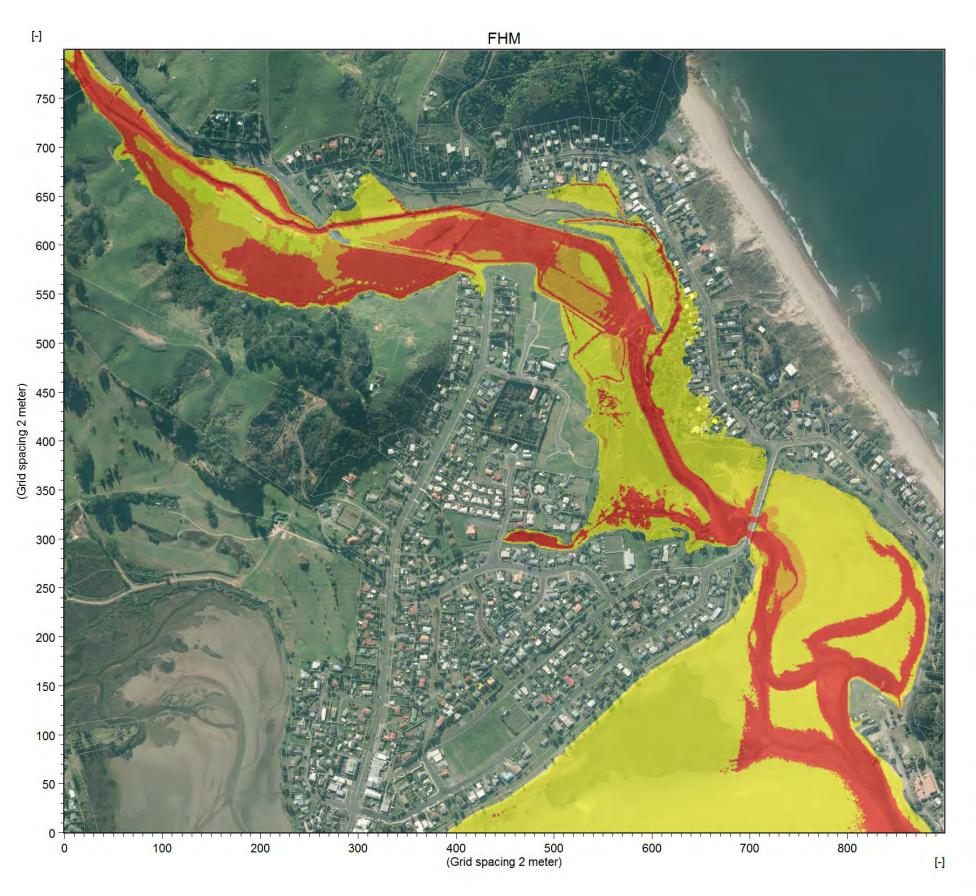
Figure A 42: Flood hazard map for proposed (partial crest) 1%AEP (100y ARI) event.
