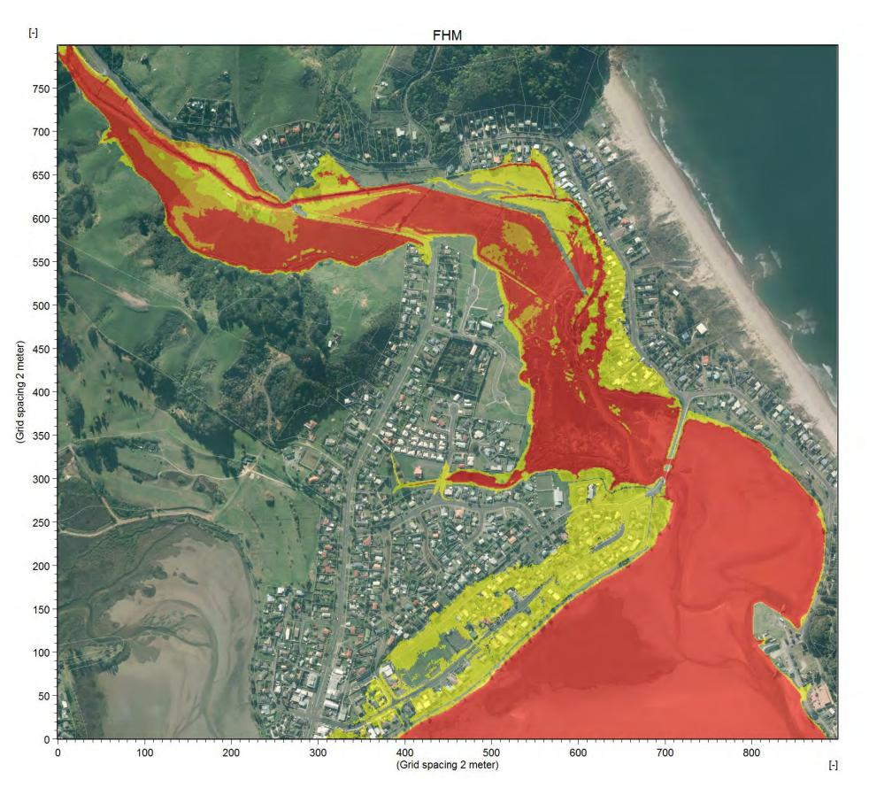
Figure A 45: Flood hazard map for proposed (partial crest) climate change 1%AEP (100y ARI) including 0.8m sea level rise event.
