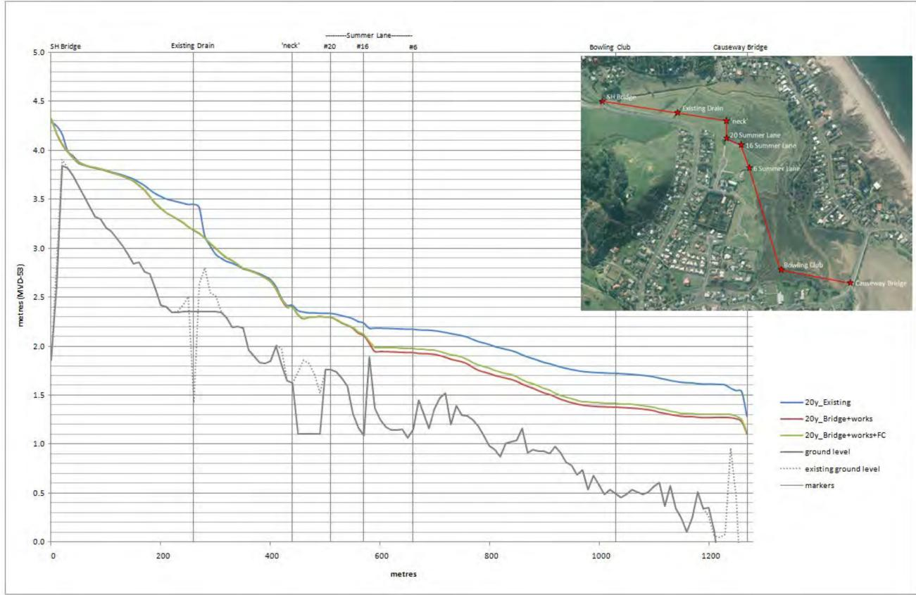
Figure A 36: Right bank floodplain maximum flood level profiles for existing, current scheme works (partial stopbank), and proposed future works (full stopbank -FC) – 5% AEP (20y ARI).
