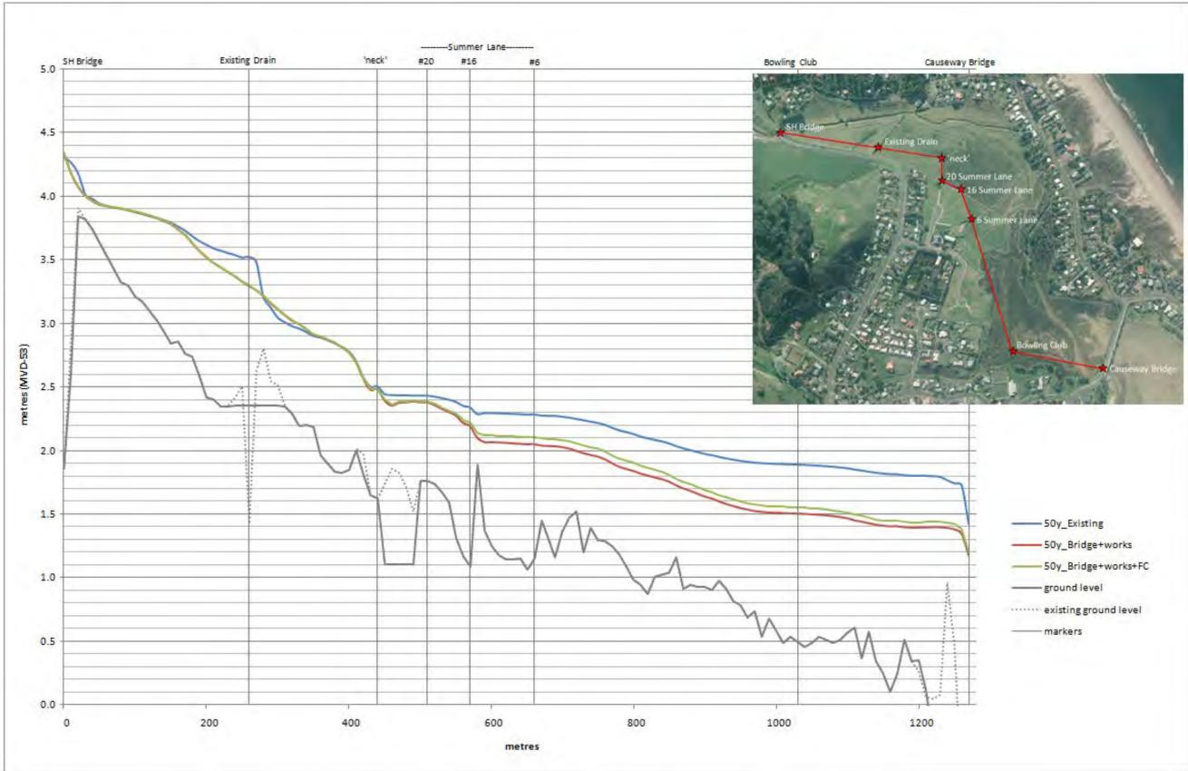
Figure A 37: Right bank floodplain maximum flood level profiles for existing, current scheme works (partial stopbank), and proposed future works (full stopbank -FC) – 2% AEP (50y ARI).
