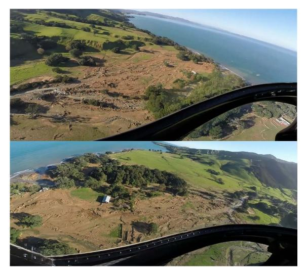
Figure 12: - Ongohi Stream floodplain debris and silt deposition
