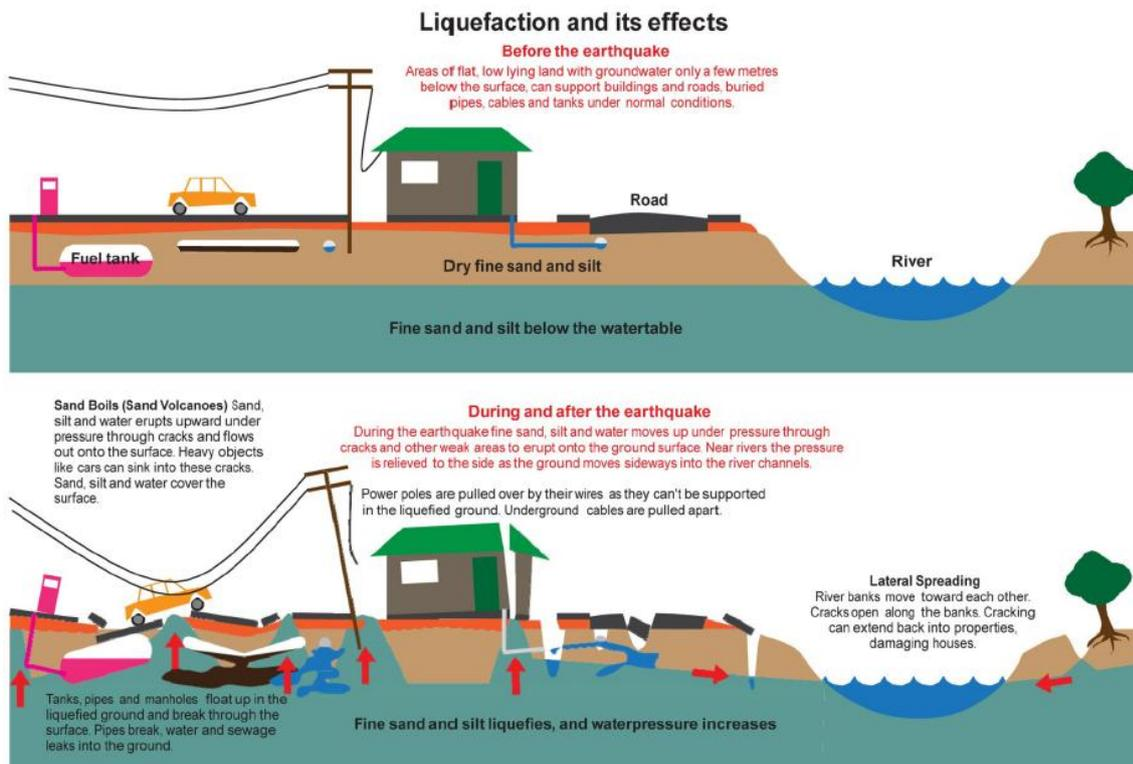
Figure 10: Liquefaction and its effects (Saunders & Berryman 2012)
