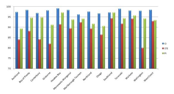
Figure 51: Condition index (CI), smooth travel exposure (STE) and pavement integrity index (PI) by region (2011)<sup>135</sup>
