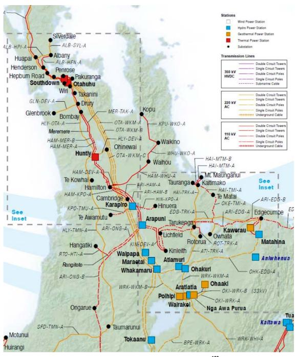
Figure 62: Transpower transmission map of the Waikato region 166
