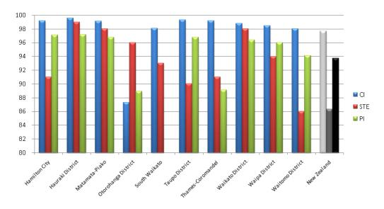
Figure 52: Condition index (CI), smooth travel exposure (STE) and pavement integrity index (PI) by TA (2011)<sup>136</sup>
