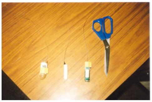
Figure 17: Different types of transmitters for use in tracker fish
