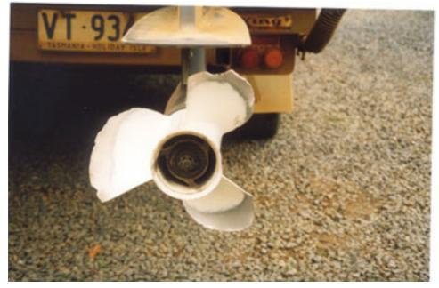
Figure 29: Propeller damage - IFS boat, Lake Crescent
