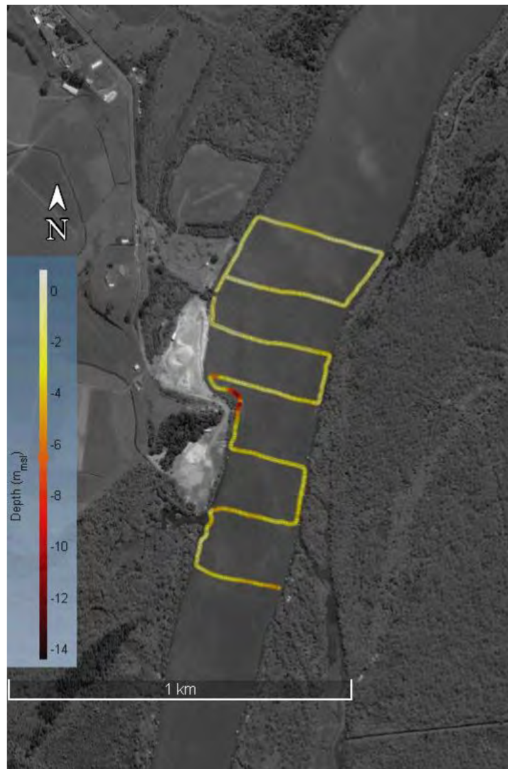
Figure 3.3: Processed survey data points at the Elbow Road site, Waikato River estuary. Depths to Moturiki MSL.
