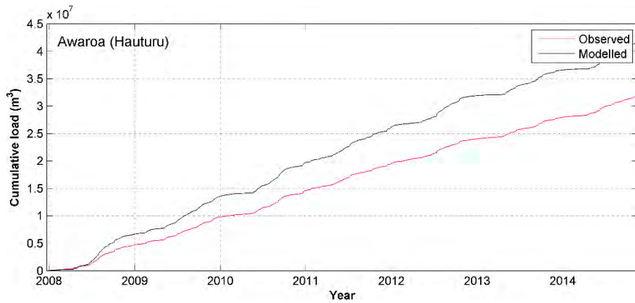
Figure A.1. Awaroa catchment sensitivity analysis using Hauturu rain gauge input: observed Awaroa cumulative water load against INCA-N catchment-modelled Awaroa cumulative water load between 2008 and 2014. By the end of the model the cumulative load was overestimated by 30.3%.
