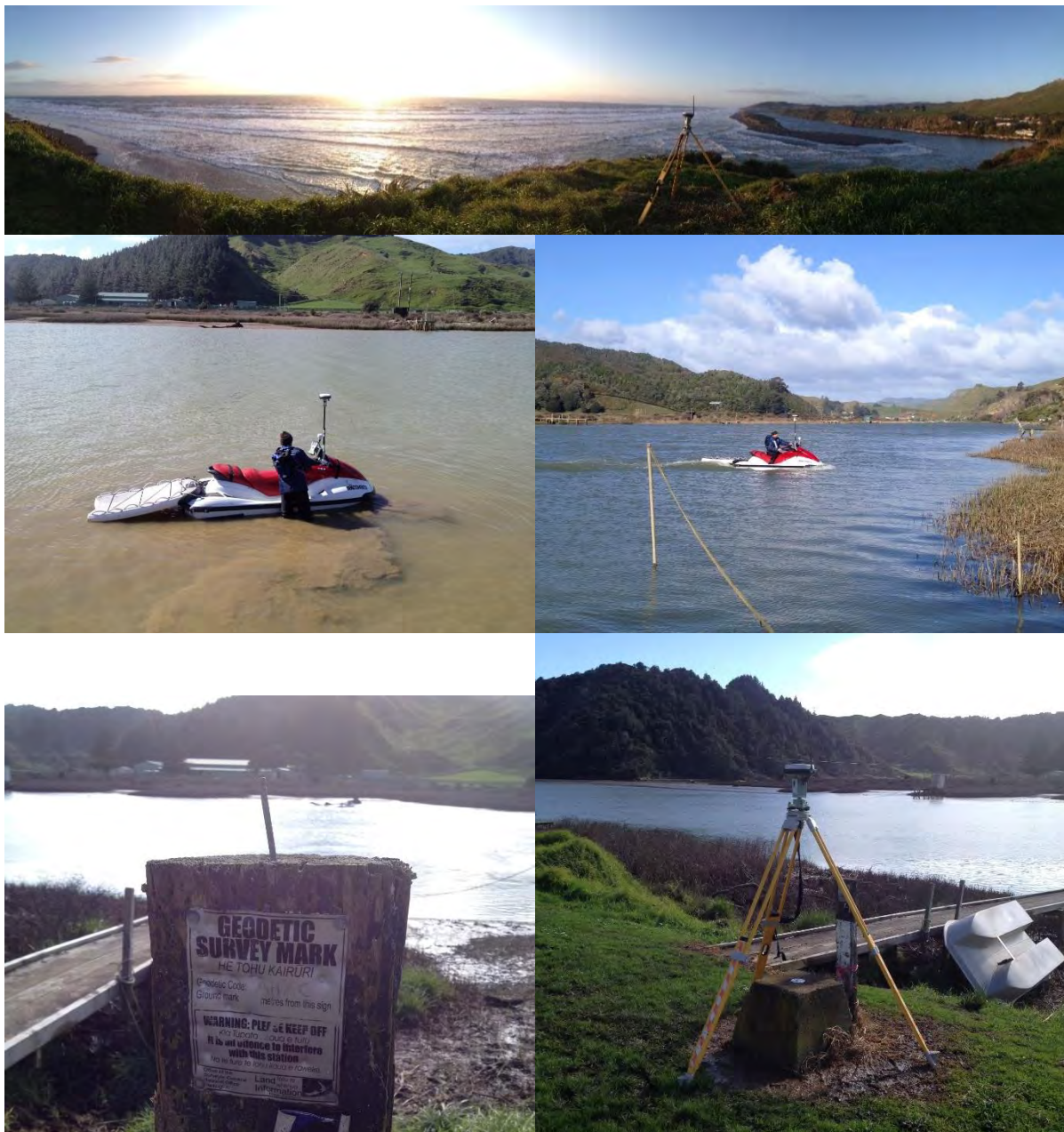
Figure 3.1: Selection of images from work undertaken at Awakino River estuary: Top, RTK Base Station established at Awakino Heads overlooking the bar, entrance and lower reaches; Middle, eCoast's Red Rocket being prepared for (left) and undertaking (right) survey work; Bottom, RTK Base station set up over a geodetic survey mark in Awakino township
