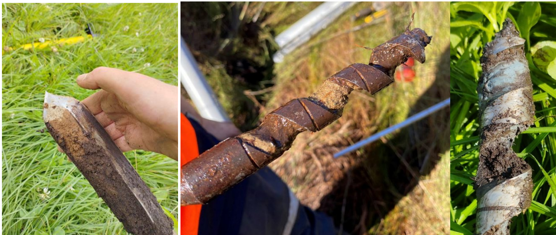
Figure 41. Examples of the transition between peat and subsurface material. Note the light-coloured material in the auger tip (left-hand photo) and peat probe tip (middle and right-hand photos), this is not organic material. However, the darker material further up the auger tip could be, perhaps with a relatively low carbon content.
