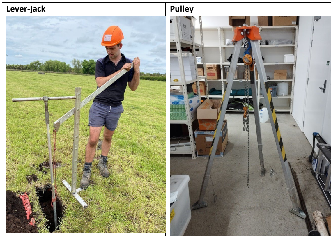
Figure 5. Photos of setup lever jack (left) and pulley system (right) used for extracting stuck peat probes. The lever jack could also lift the peat probe at the handle.
