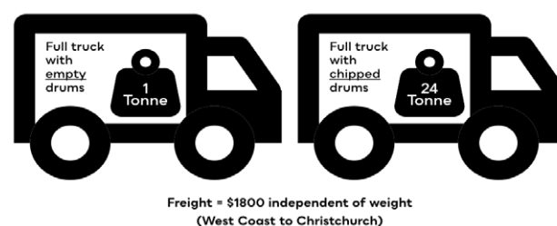
Figure 2: Freight comparison of shipping empty 200 litre reusable drums versus shipping compressed plastic (reported by a business participant)
