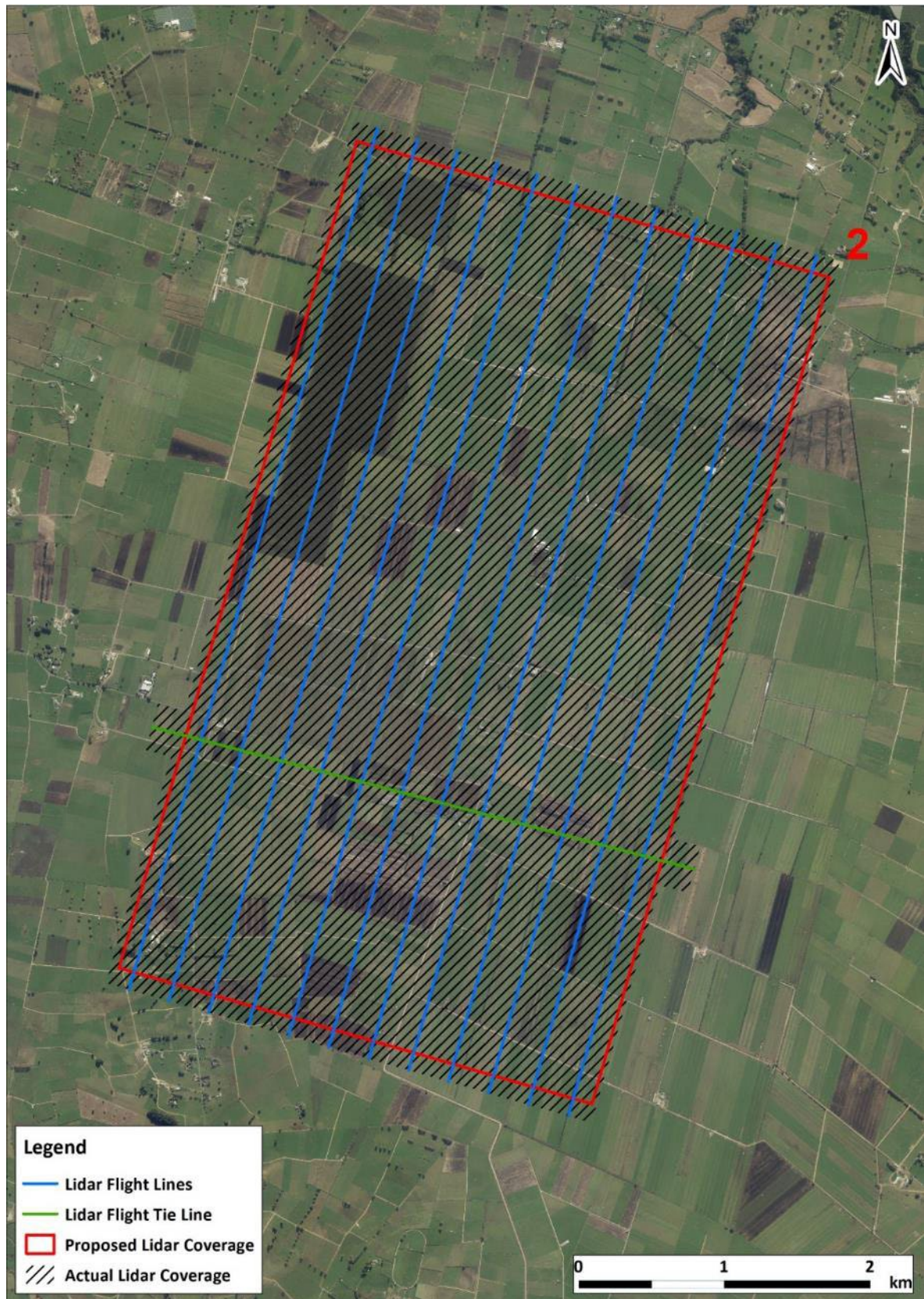
Figure 3. Example of flight lines and actual LiDAR coverage area from Moanatuatua, which was flown second (see Fig. 2). LiDAR flight lines, in blue, were flown along the longest axis to minimise turning time, and then a perpendicular flight line, in green, was carried out at completion to tie all flight lines together. LiDAR captured from each flight line overlapped the next, and actual LiDAR coverage, indicated by the black lines, was slightly larger than the proposed area, shown as by the red polygon.
