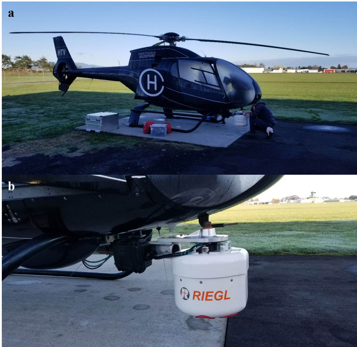
Figure 4. (a) Airbus EC120 being prepared for LiDAR flights on 28 April 2021 at Hamilton Airport, (b) LiDAR sensor array mounted in an enclosed pod and carried on a forward mounted boom.
