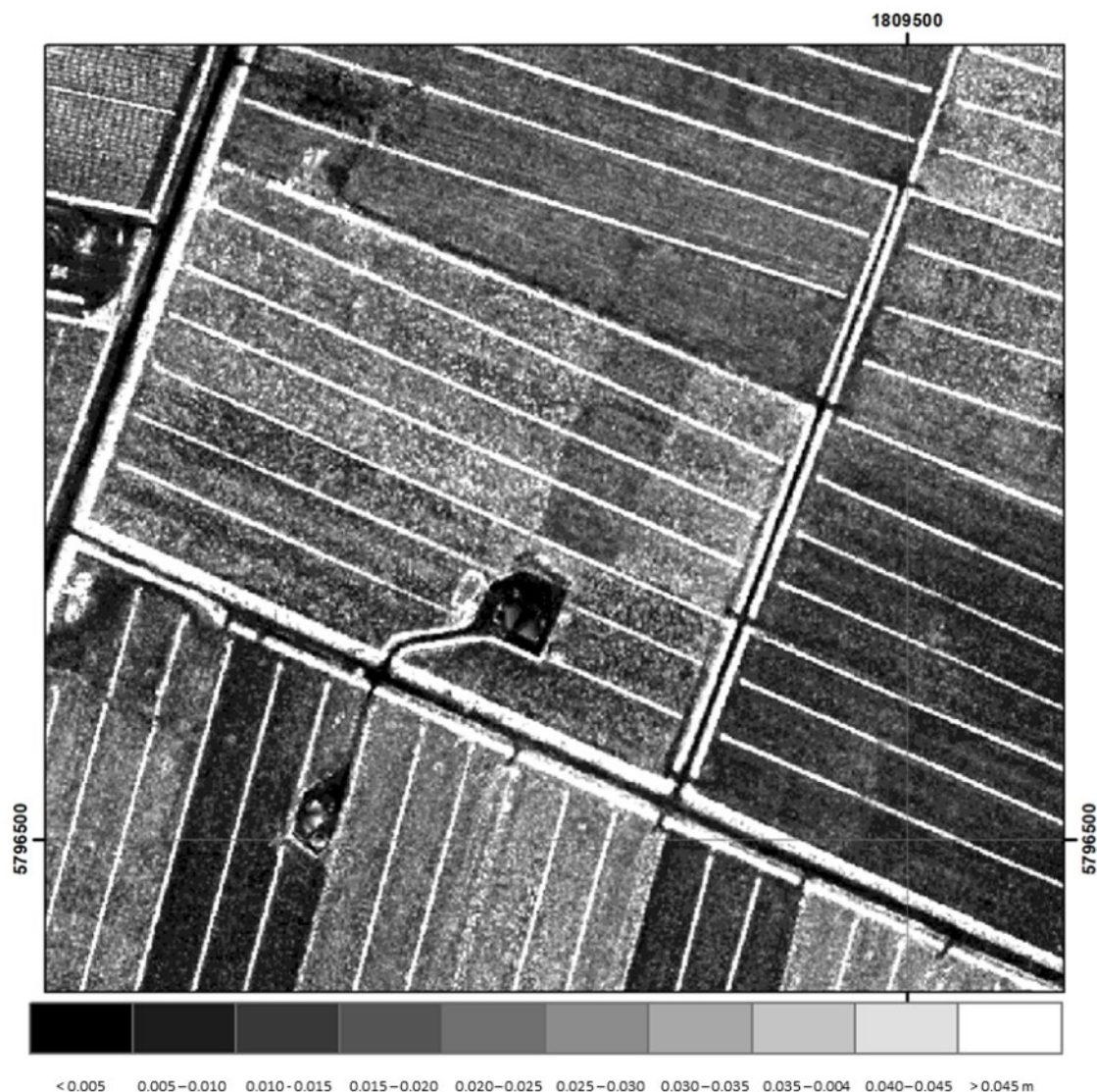
Figure 10. Detrended SD of elevation of the ground returns calculated at a 0.5-m grid sampling for the Moanatuatua LiDAR testing flown in June 2019. Shorter pasture is characterised by low SD of elevation (darker colours), while longer pasture (rougher surfaces) have higher SD of elevations (lighter colours).
