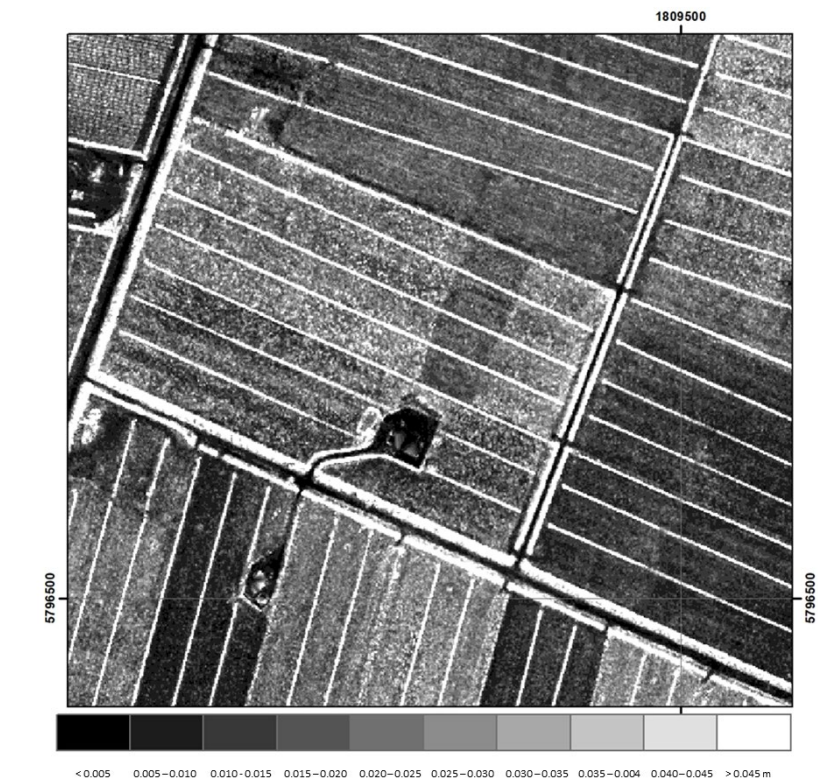
Figure 8. Detrended SD of elevation of the ground returns calculated at a 0.5 m grid sampling for the Moanatuatua survey data. Recently grazed (short) pasture is characterised by low SD of elevation 0.005 – 0.01 m, while longer (rougher) surfaces have higher SD (0.04 – 0.05 m).
