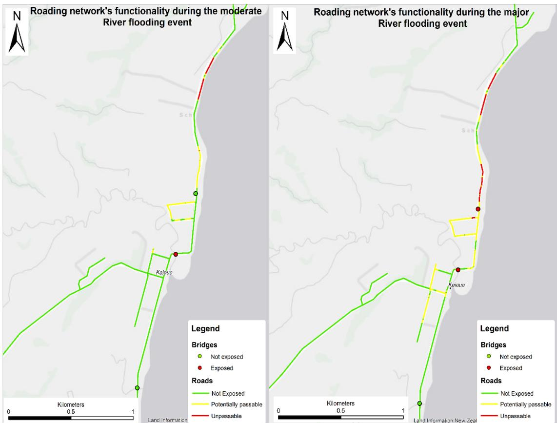
**Figure 49 Exposure of roads and bridges to Haurahi Stream flooding in compartment 2 (note: potentially passable is <0.5 m flood depth; unpassable is >0.5 m flood depth)**
