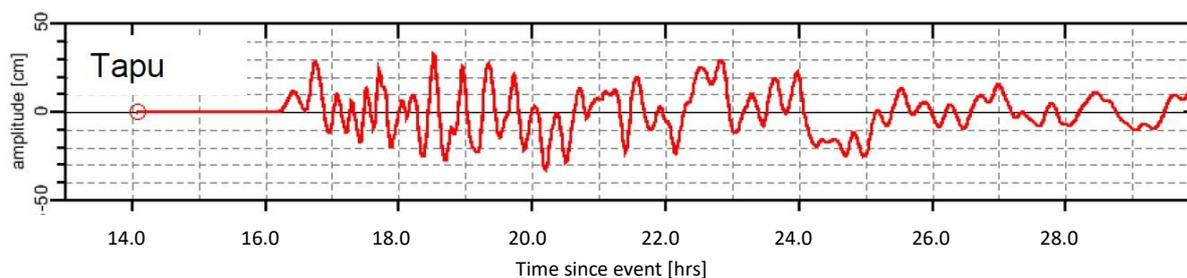
**Figure 10: Wave arrival times and inundation levels from the 'FF 7' distant source scenario**
