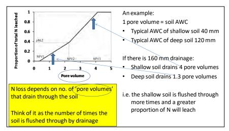
**Figure 1**. Shape of N leaching curve as derived by Cichota et al (2012). NPV ('number of pore volumes') values denote start of leaching (nPV1) an inflexion in the linear relationship between pore volumes drained and proportion of N leached (nPV2) and number of pore volumes required to complete leaching (nPV3). These values vary with soil type
