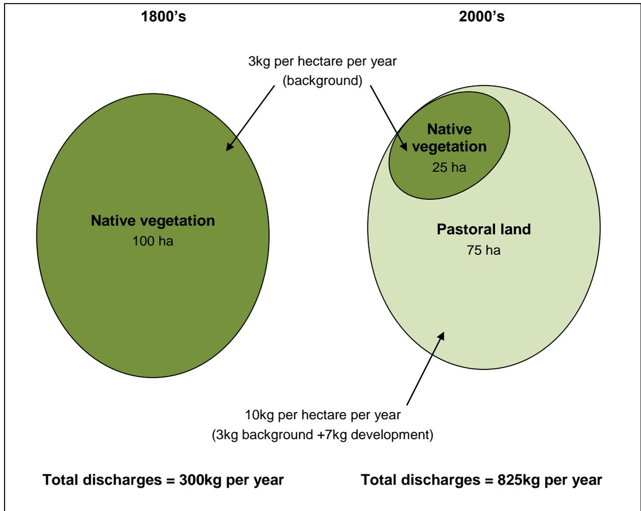
**Figure 1: Example of natural background discharges and increases from development**
