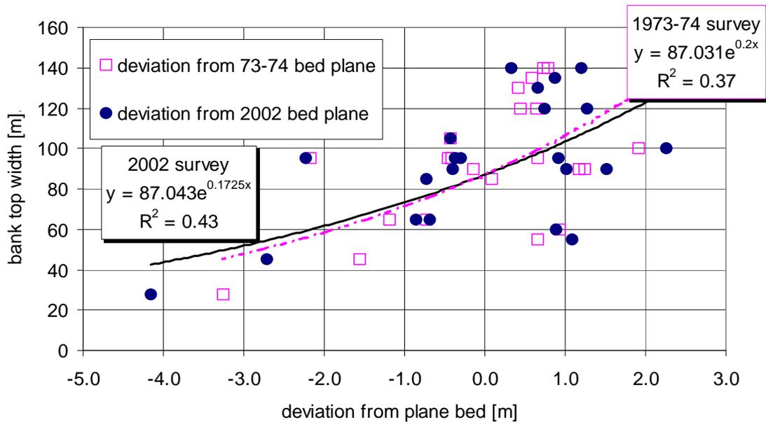
**Figure 21 Relation between bed level and bank width.**
