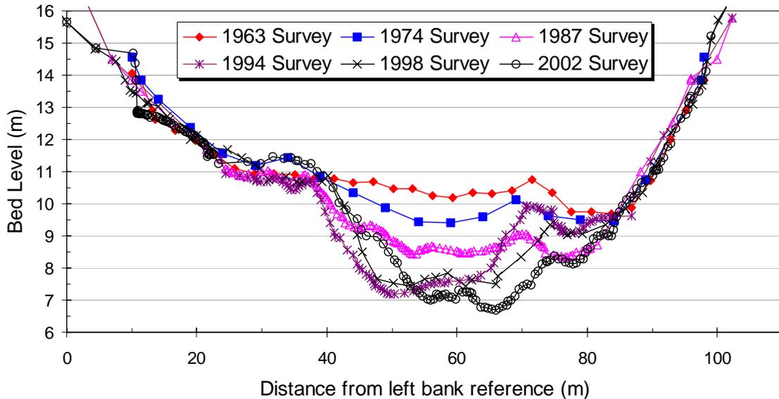
**Figure 15 Cross section 151 at Hamilton's Victoria St Bridge showing evolution over time. Vertical scale is 10 times the horizontal scale.**
