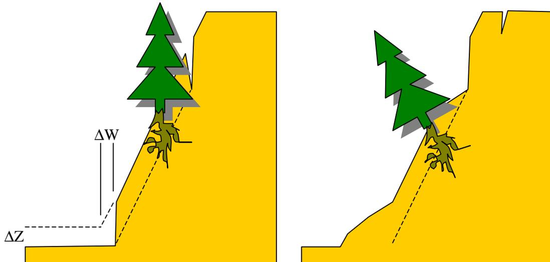
**Figure 13 Schematic representation of bank failure by bulk sliding showing: degradation  $\Delta Z$  and widening  $\Delta W$  (left) and situation after failure (right).**
