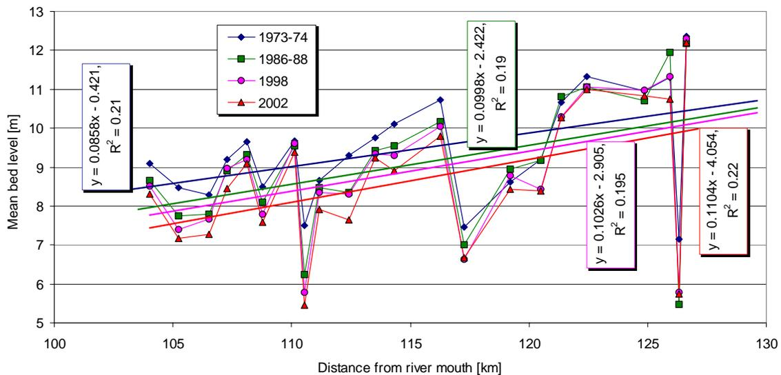
**Figure 19 Trends in mean bed level of 22 Hamilton cross-sections. Trendlines represent a plane bed smoothed of local humps and hollows.**
