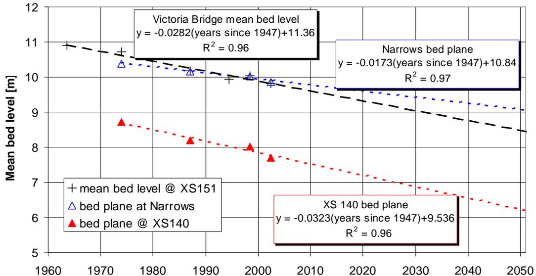
**Figure 20 Trends in mean bed level at Victoria St Bridge (XS 151) and trends in level of the bed plane at Pukete Boat Ramp (XS 140) and downstream of Narrows Bridge (km 126), extrapolated to 2050.**
