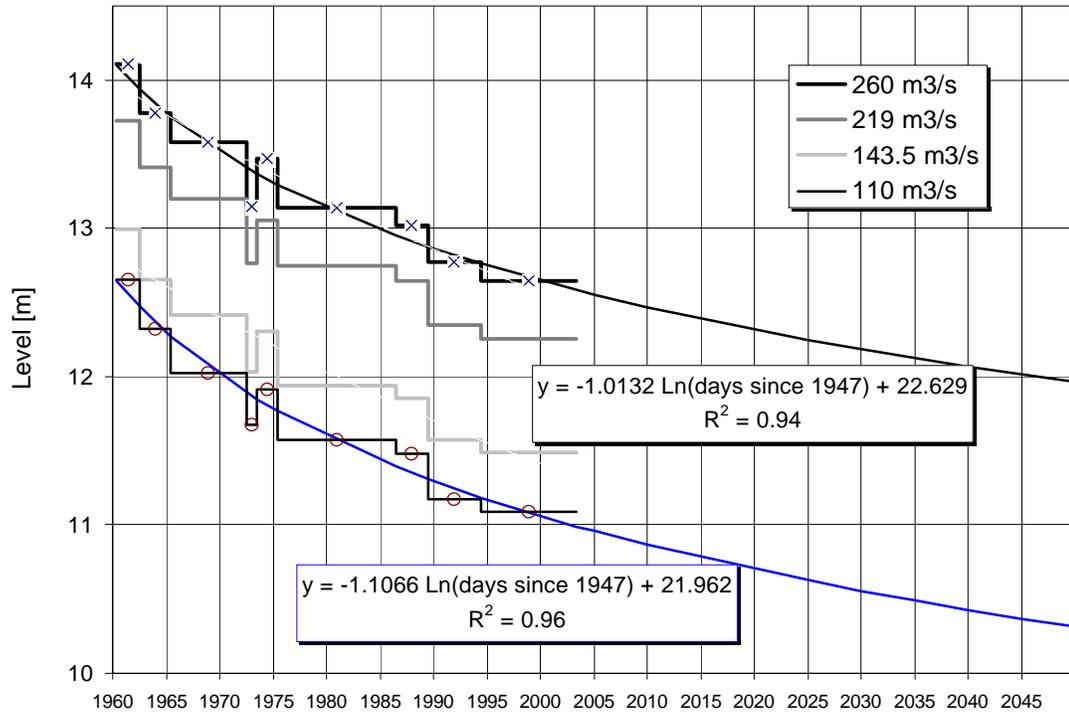
**Figure 17 Victoria Bridge specific gauge record extrapolated to 2050**
