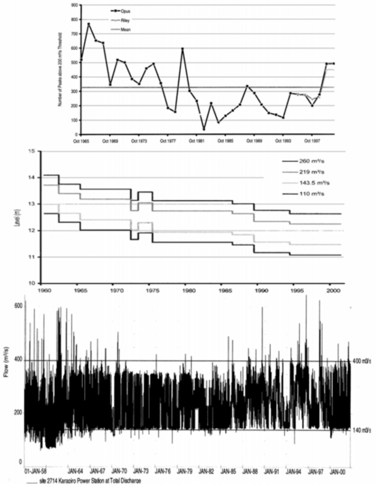
**Figure 16** Aligned time series from Freestone Evidence showing: Number of peaks per annum above 200 m<sup>3</sup>/s for Karapiro half hourly outflows (top), specific gauge record for 4 flows at Hamilton's Victoria Bridge (middle) and Karapiro discharge (bottom).
