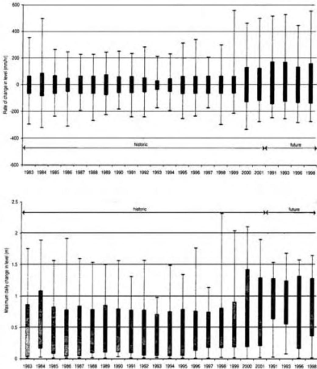
**Figure 14 Historic and future water level variation 400 m downstream of the Narrows bridge showing statistics on rates of change [mm/hr], top, and daily range [m], bottom, as projected by Webby. Whiskers show annual maximum and minimum values, boxes show values exceeded 10% and 90% of the time.**
