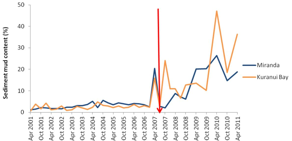
**Figure 18:** Changes in sediment mud content at Miranda and Kuranui Bay over the duration of monitoring. The red line denotes the change in analysis technique. Data were split at this point to test the statistical significance of the overall trend.
