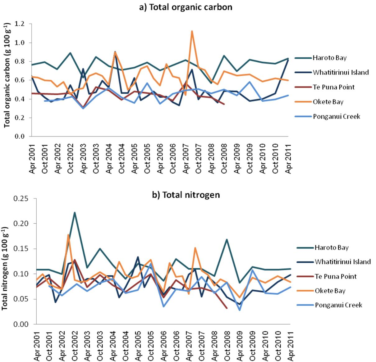
**Figure 20: (a) Changes in sediment organic carbon and, (b) total nitrogen content in Raglan (Whaingaroa) Harbour. A negative trend was detected for organic carbon and nitrogen at Te Puna Point.**
