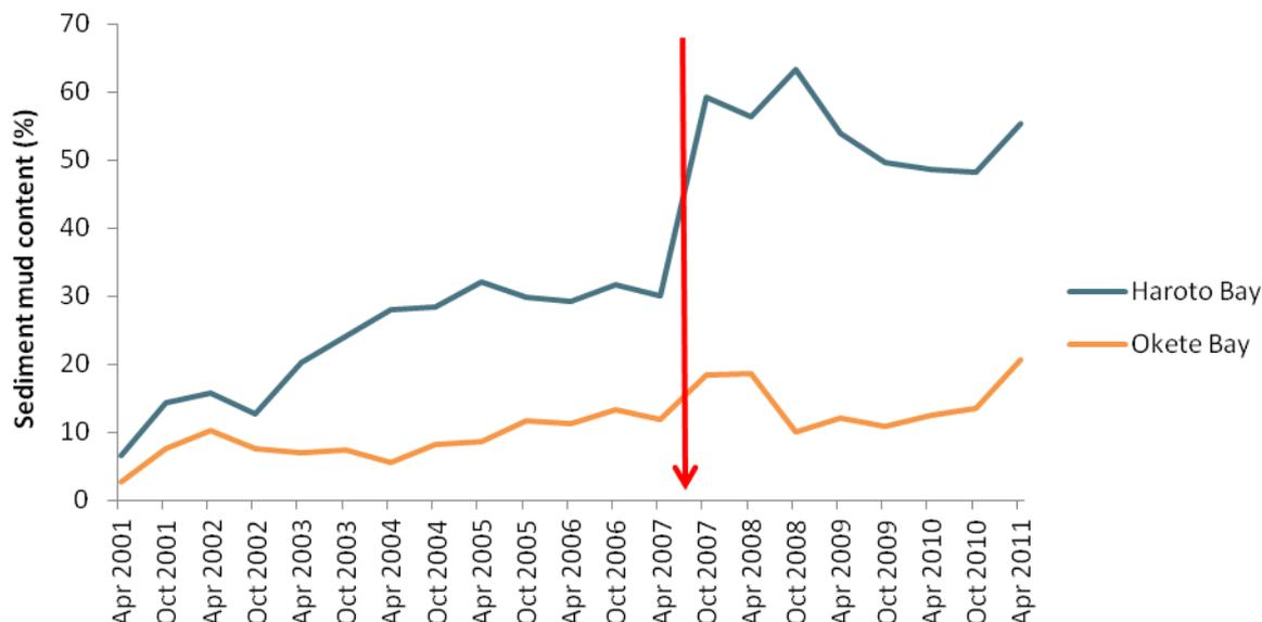
**Figure 21: Changes in sediment mud content at Haroto Bay and Okete Bay over the duration of monitoring. The red line denotes the change in analysis technique. Data were split at this point to test the statistical significance of the overall trend.**
