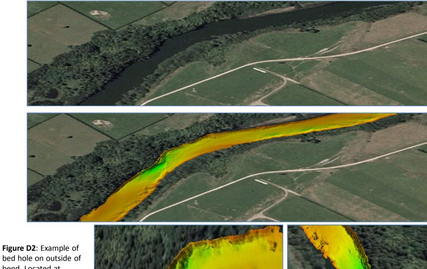
bed hole on outside of bend. Located at chainage 136.13km (160m downstream of section 169) Approximately 5 metres deep
