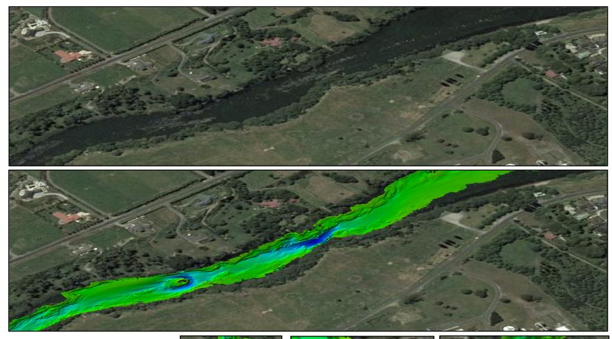
Figure D3: Example of a long hole. Located at chainage 107km (from 220-340m downstream of Section 141). Hole is over 7m deep
