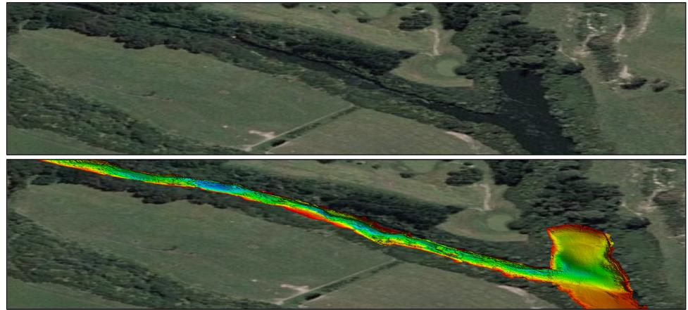
**Figure D5**: Example of a fault forming a sill. Located at chainage 144.65. The bed level drops by 8m, with individual holes a further 1.5 metres deep.
