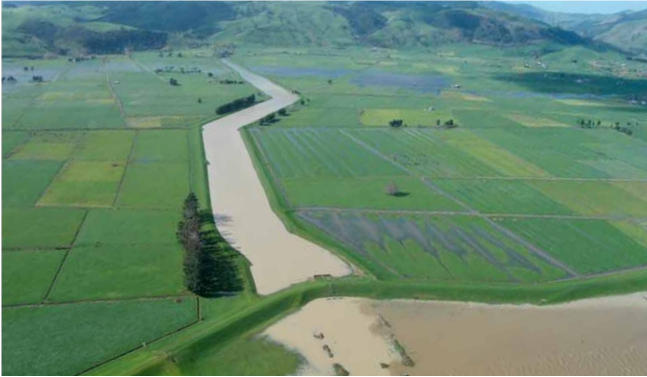
The junction of the Waihou River and Kurere Stream. The stopbanks, shown at the bottom of the photo, help protect land during flood events.
